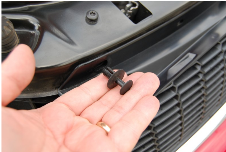
Illustration 4: A shot of the "pin" assembly removed from the top of the grille. Remove all four.
