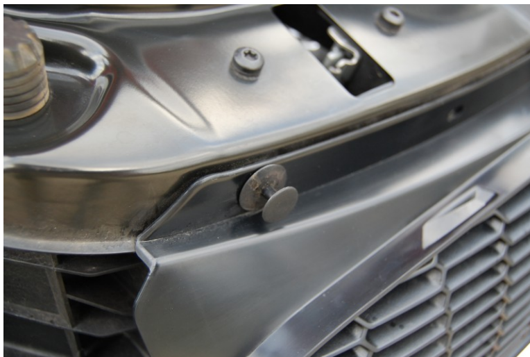
Illustration 3: A shot showing the "pin" slid out. These work like a screw anchor for sheetrock. Once you pull the pin out, the whole thing comes out.
