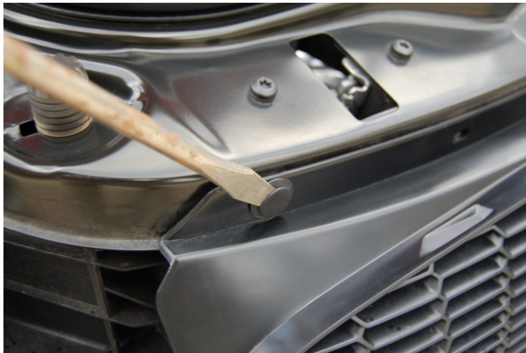
Illustration 2: I use a flathead screwdriver to pop these out. Maybe there is something better? They just slide out.
