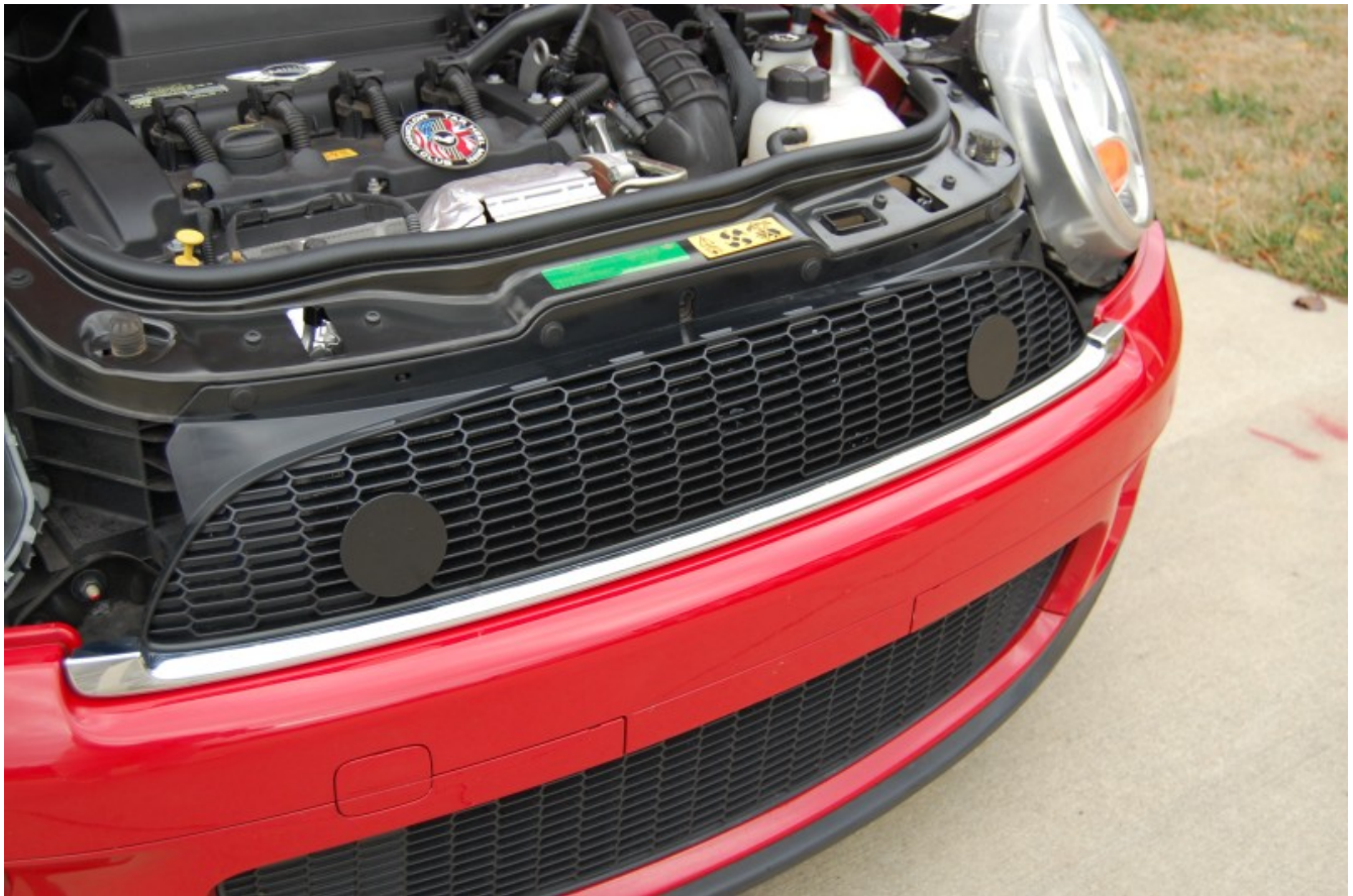
Illustration 8: Tada - two new grille badge holders installed.
